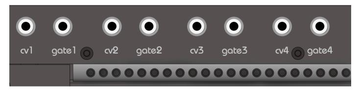
The CV outputs are used to control the frequency of VCO (voltage controlled oscillators) modules. They output a voltage that changes as you press keys on the keyboard or send MIDI notes to the device according to the 1V/octave standard commonly used in the euro rack world. The CV outputs range from 0 to + 10V allowing a total span of 10 octaves.
