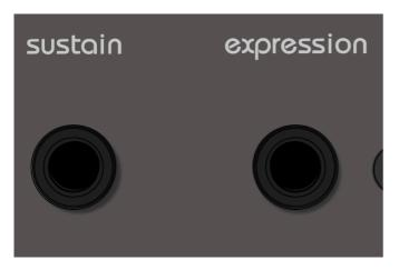
Connect a sustain pedal to the sustain input jack to trigger the latch function by foot.
