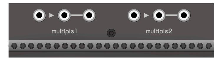
NiftyKEZ has 2 Multiples named multiple1 and multiple2. Both have identical functionality. Multiples take an input signal (jack1) and replicate the same signal at the 2 outputs (jacks 2 and 3). A multiple is useful for sending the same signal to several modules.
