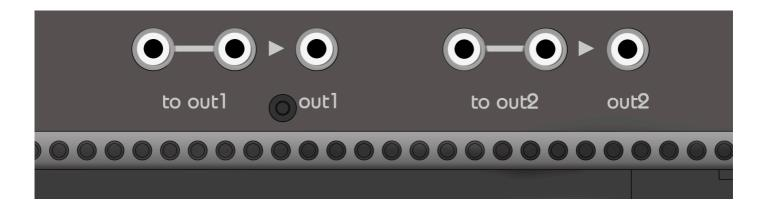
The **to out1** jacks can also be used as a summing circuit, since the **out1** 1/8" jack outputs the sum of the 2 signals patched to the **to out1** jacks.
